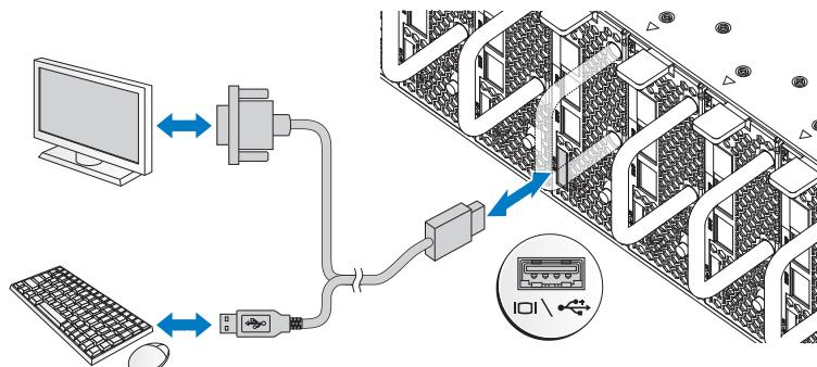
The connector on the front of your system has an icon indicating which cable to plug in. Connect a keyboard, mouse, or monitor (optional).
